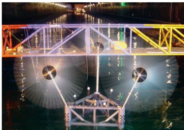
Proof of concept – model tests in wave basin have shown that the WindSea concept is up to the task of performing in the harsh offshore wave environment (photo: WindSea)
